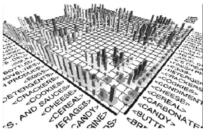
Fig. 25 MineSet's association rule visualizer [62] maps rules to the x- and y-axes. The confidence is shown as the bars and the support as the bars with discs
